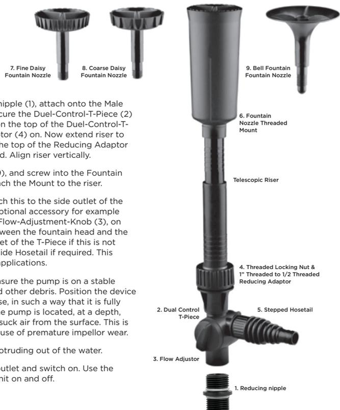
Using the 1" to ½" threaded reducing nipple (1), attach onto the Male Threaded outlet of the pump. Now secure the Dual-Control-T-Piece (2) onto threaded reducing nipple. Now on the top of the Dual-Control-T-Piece (2), connect the Reducing Adaptor (4) on. Now extend riser to the desired height, then secure onto the top of the Reducing Adaptor with the threaded locking nut provided. Align riser vertically.
