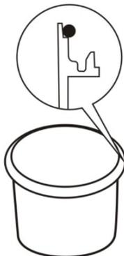
Firmly push the lid back onto the canister. Fasten the lid clamp in place and reconnect the inlet and outlet hoses.
