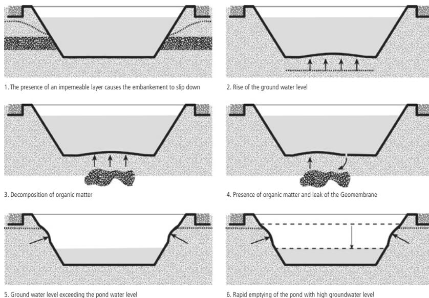
Fig. 3 : Some causes of excessive pressure
